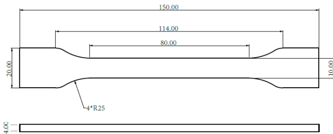
Tensile testing specimen; ASTM D638 (ISO 527, GB/T 1040)
